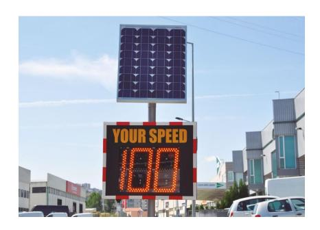
SP-SSD is a solar powered speed meter system developed to inform drivers of their actual speed. It have a CW Doppler Radar that detects vehicles up to 199Km/h(123Miles/H). Has a range of detection up to 180M/590Ft and can detect multiple vehicles as well
