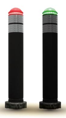
SP-PCLB<sup>TM</sup> has been developed thinking about distracted walkers. The light on the top of the bollard is at the angle of view of a pedestrian who is looking at a cellphone. Connected with the pedestrian crossing traffic lights, the LED on top of the bollard changes from red to green – according to the pedestrian crossing traffic lights -, alerting pedestrians if it is safe to cross the street or not.
