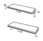
Step 3. Adjust the LED light to the Angle you need, and then fix the installation area with screws
