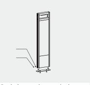
2. Set the lamp on the mounting base plate, fix the screws on both sides, and finally block the screw hole with a plug.
