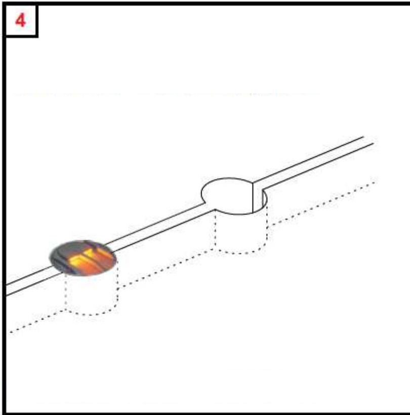
4. Align the tubing and the “boxed out” shells at the proper orientation so as to allow for the wiring to connect to the shells.
