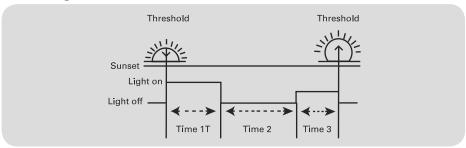
The ON and OFF functions are how the light is controlled. The light is turned on at dusk with a pre-programmed setting function and works until dawn. The lights are controlled automatically by the built-in charge controller with light sensitive timings. At sunset NTTV (Night Time Threshold Voltage) goes less than 7 Volts from the solar panel, the lights will turn ON. In the morning the DTTV (Day Time Threshold Voltage) from the panel reaches 7 Volts the lights will turn OFF.
