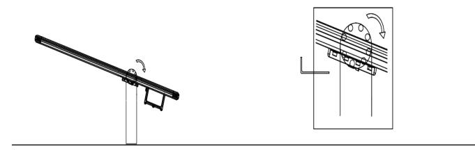
2. Fix the led module to the small u-bracket with 4 screws for each one, rotate the lighting angle to illuminate area.
