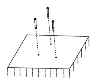
3. Place bracket as per below drawing, match the location of holes and fix it with screws.
