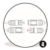
Connect the MC4 Connectors to the Solar PV panel.
