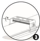
Using a screw driver, secure each clip onto the SP-XL with the Tension bolt. Note: This is only to secure the SP-XL so it cannot be removed - Do not over tighten.
