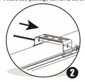
Insert Tension Bolt and attach the SP- XL to the metal clips.
