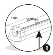
Connect the two metal clips into position and attach to the surface. It is recommended that each clip is positioned approximately 7.8in from each end of the SP-XL Caution: Ensure correct anchor sleeves are used for surface material. Please see package contents before installation.
