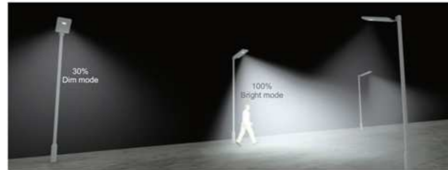
Solar lights stays dim when humans are not around but increase its luminosity when it senses signal that people walk nearby.
