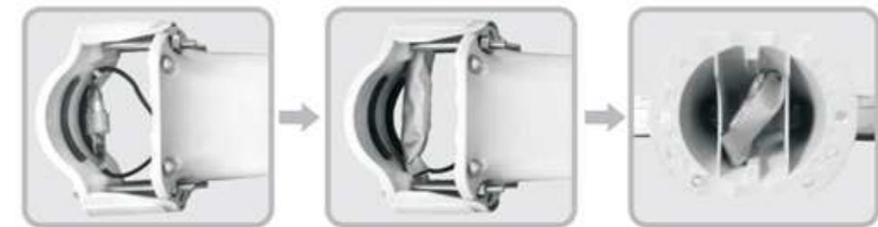
Connect the waterproof wire terminal clamps. ( Figure 2 )
