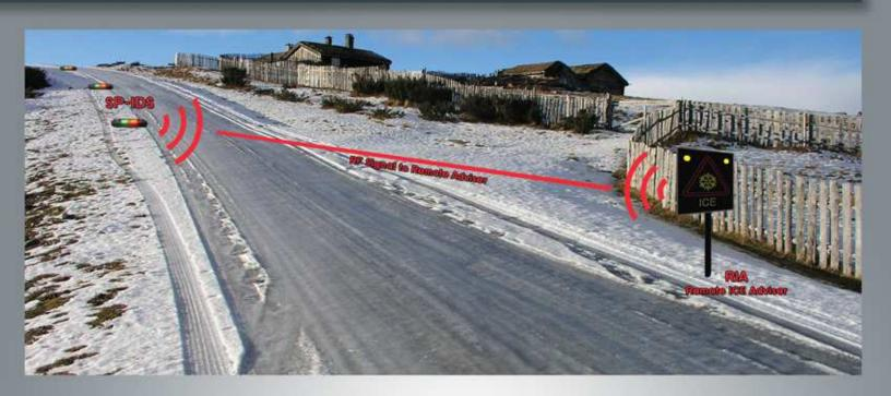
Very powerful ice detection system with humidy sensor and an intelligent temperature reader. The system works with solar energy, allowing the placement of this system in any critical point of a road.
